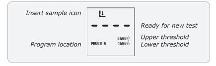
The display shows the **PROG** number, the program upper  $(\uparrow)$  and lower  $(\downarrow)$  thresholds, and the total number of test results stored in the memory (e.g. 47).
