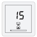
**NOTE:** During self-calibration, there must be no CariScreen Swab device in the unit and the lid must remain closed. If the <u>L1</u> icon is shown with the arrow flashing, open the lid and remove the CariScreen Swab device from the unit. If the <u>L</u> icon is flashing, close the lid.
