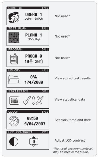
Use the (A) and ( $\forall$ ) buttons to scroll through the menu list, and then press the ( $\circledast$ ) button to select the required menu option, or the ( $\circledast$ ) button the exit the menu.
