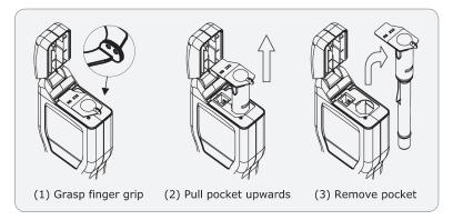
**CAUTION:** Great care should be taken when removing the pocket not to damage it or the surrounding casework. Do not use excessive force. Never use a tool to pry the pocket out.
