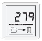
To accept and start the erase function, press and hold down the  $\bigcirc$  button for 1 second, or press any other button to exit the option.
