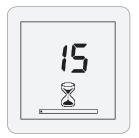
**NOTE:** For consistent results, always keep the unit upright and steady while it is performing a measurement to ensure that the liquid in the CariScreen Swab device is at the bottom of the tube.
