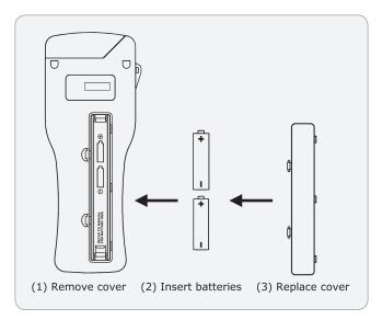
**CAUTION:** Be careful not to insert the batteries backwards, as this may cause permanent damage to the unit's electronics. When the batteries are inserted correctly, the unit automatically
