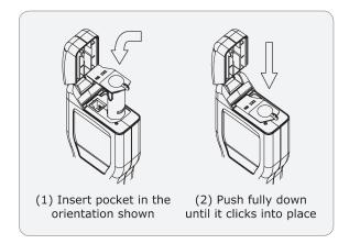
**WARNING:** Do not use excessive force when replacing the pocket. If the pocket jams during insertion, remove it fully, check for obstructions or damage, and then try again.
